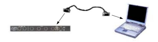
Selecting COM1 - 4 enables communication with the LMS244; the Main Menu appears with Connected and the COM Port Number shown in the bottom left hand corner of the menu screen.
