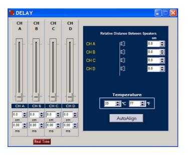
In this window, you can configure the final delay to each way. To do this you have sliders that allow you to adjust the various delays in the outputs on steps of minimum samples. By modifying any of them, the value of the delay in centimetres and in milliseconds will be displayed below. If you are fine-tuning delay setup, you can enter to the indicators and increase or decrease with the keyboard up and down arrows.
