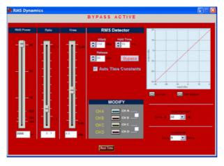
The adjustment of the parameters of the dynamics will be vital for the safety of the loudspeakers. Not only Power threshold, but also the **Hold Time** and **Release**, because depending on these parameters more or less peaks will be passing on the RMS Power threshold.
