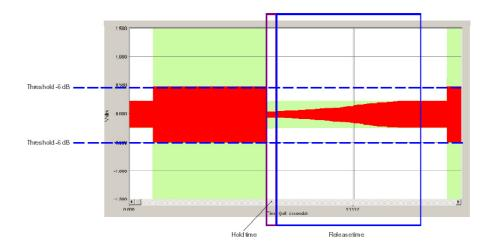
When the input signal exceeds the threshold limit set (-6dB in this example), dynamics start working by reducing the signal to the threshold. The difference with the RMS limiter (see page. 29) is that the Peak limiter has no time attacking, since it is instantaneous and does not let any transitional signal above the threshold we have set.
