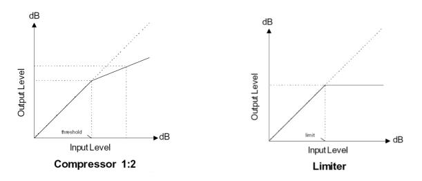
In the **Compressor**, the **Output** signal follows the **Input** signal if you are below the threshold. Once it exceeds, the output is mitigated depending on the chosen **Ratio**. In the next graphic there is a 1:2 ratio, which means that once the signal exceeds the threshold for every 2 dB increase in the input we will have 1 dB increase in the output. The limiter works like a compressor with 1: $\infty$  (infinite) Ratio, not leaving to the output level exceeds the threshold.
