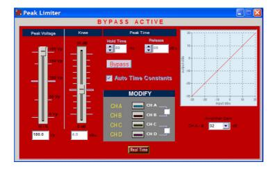
By default, when you connect a S amplifier with DSP module to the software, both limiters, RMS and Peak, are **Bypassed**; so if you want to configure the limiters you have to click Bypass button in order to introduce the parameters to fix the limiters.
