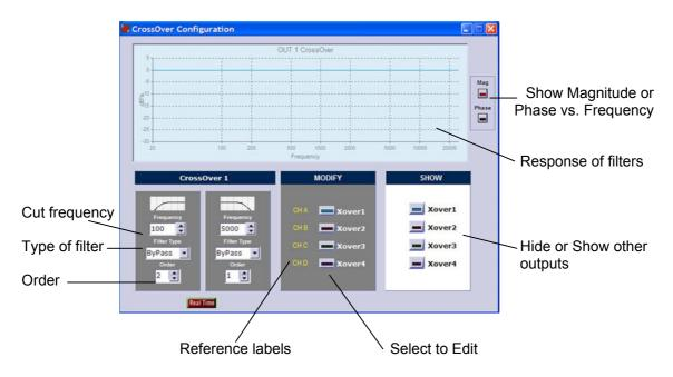
The two columns represent the low cut (**High Pass Filter**) and higher cut (**Low Pass Filter**) in which you can configure crossover frequencies, the type of filter used for CrossOver and order of each filter to adjust the slope.
