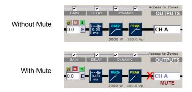
You can adjust **Output Gains** for example: in order to get the right signal to each of the connected amplifiers, according to their own input sensitivity. And/or to compensate electrically the different ways depending of the sensibility of the transducers in a multi way system, knowing that most of the times High and Mid frequencies needs an acoustical adjustment.
