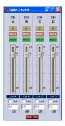
By default all Gains appear at 0 dB. We have +6 dB of gain and -30 dB of attenuation, in increments of 0.1 dB. You can use the sliders, or if you w ant a precise control you must use the keyboard arrows up and down, t o go from 0.1 dB of 0.1 dB..
