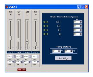
We also have the **AUTO-ALIGN** button, which will internally calculate times, and automatically adjust all the delays required to leave the system in phase.
