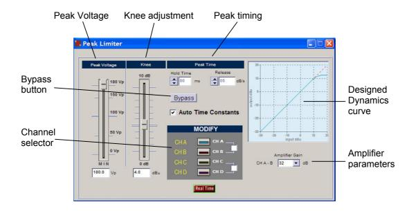
As in the screen of RMS Dynamics, if we do not want the **Peak** limiter to work, we can press the **Bypass** button to disable this action. Then the Peak Limiter screen will look like this:
