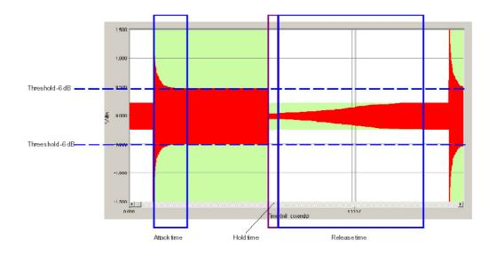
When the input signal exceeds the RMS Power threshold compression/limiting fixed, dynamics start working, reducing the signal to this threshold. The amount of time this transition lasts is the **Attack** time.
